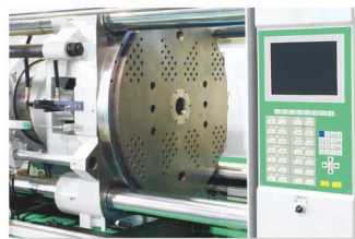
● 直壓式鎖模結構 Hydraulic Clamping Structure
